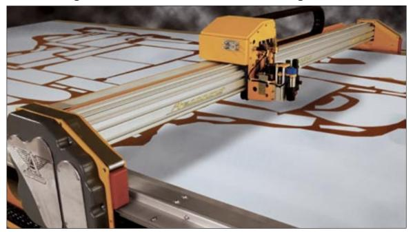
The Aeronaut Leather System is a complete system for cutting leather comprising automated pattern and hide scanning, interactive nesting and computer controlled cutting.
